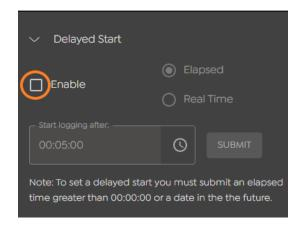
Enable Delayed Start by checking the checkbox.
