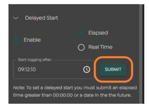
Press the Submit button to send the elapsed timer settings to the logger.
