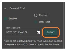
Press the Submit button to send the Real Time settings to the logger.
