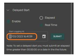
The date/time delay can also be directly entered by clicking on the 'start logging at' time and typing valid values.
