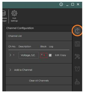
On the right side of the display, click on the Channel Configuration tab Configure at least one channel as described in 4.6.3 of the user manuals.
