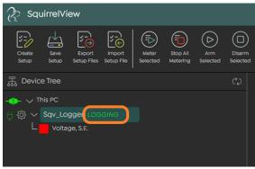
When the Delayed Start timer conditions are met LOGGING will be displayed, informing you that the logger is recording data.
