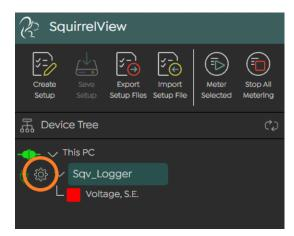
To configure the logger for delayed start, click on the icon associated to the logger to open the logger settings:
