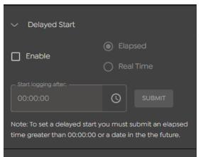
Scroll to the bottom of the tab's window, until the Delayed Start settings are displayed. (by default these will be disabled)
