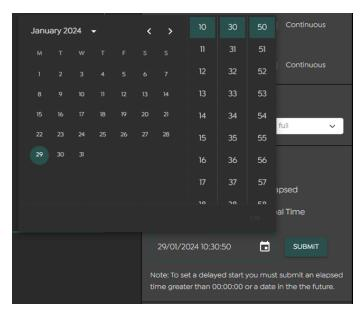
The Real Time selection window will open, click on the date and time to set the delayed start time.
