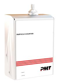
The 9301 and 9501 PoE particle counters provide a range of particle size measurement from 0.3 to 25.0  $\mu$ m at a flow rate of 0.1 CFM (2.83 LPM). These sensors allow for efficient particle counting with specifications that exceed the ISO 21501-4 and JIS B9921 calibration standards.
