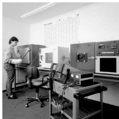
Temperature testing facilities for Höntzsch proximity switches
