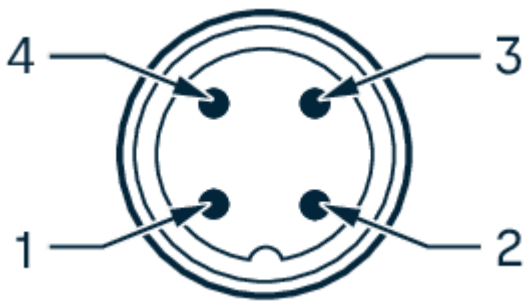
M12 4-pin A-coded female connector pinout
