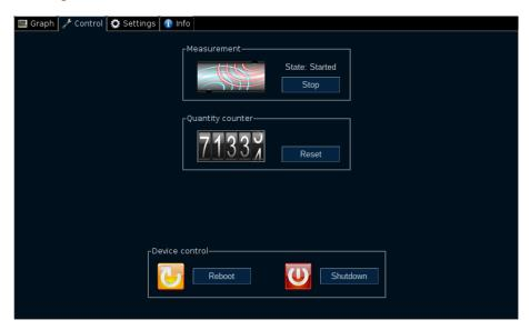
In Tab Control the measurement can be paused. The graph is no longer updated when the measurement function is stopped; the last measured value is permanently displayed. The measurement data via TCP interface also no longer change, the last measured values are always transmitted. The analog output is also frozen at the last value.
